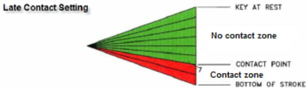
Set the key to make contact earlier in the downstroke.
