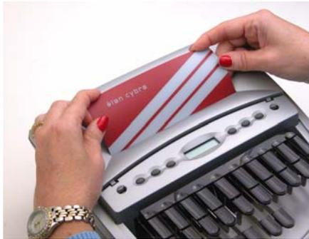
3. Push the top gently to slightly bow the nameplate and insert the top into the top of the nameplate frame.
