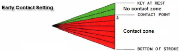
Set the key to make contact later in the downstroke.
