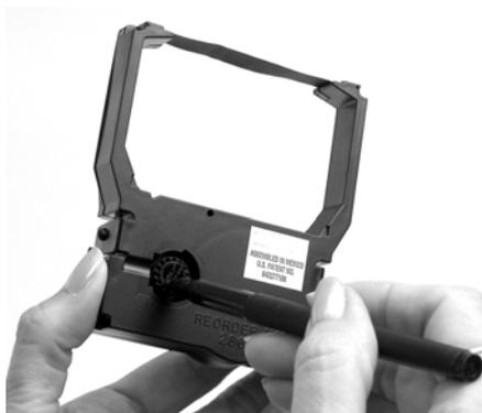
6. Press the number bar down with one hand. With the other hand, squeeze the cartridge handles and insert the new cartridge into the Stentura Protégé, placing the ribbon between the row of type bars and the platen.
