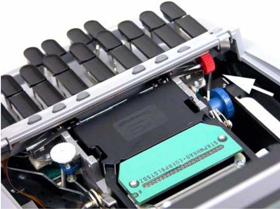
To adjust the depth of stroke:
